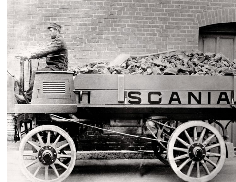
Scania's First Truck, dating from 1902, carried 1.5 tonnes of cargo and was equipped with a 2-cylinder 12 hp engine placed under the driver's seat.
